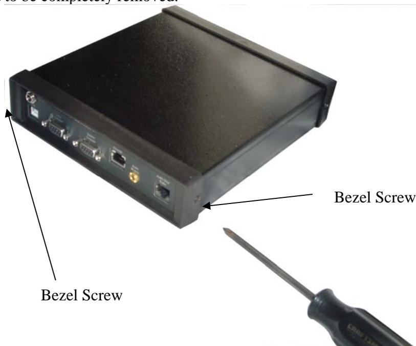
3. Remove the bezel and locate the four back panel screws. Remove them.
